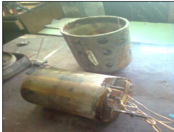
Fig. 7. Antenna after insulated
